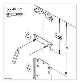
Retaining plate C should only be used if dimension Y is greater than 14  $^{3/}_{8}$ " (365 mm.) It provides additional stability for the chimney extension.
